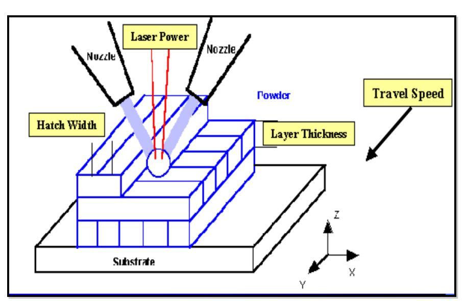
Figure 1. M-LAM deposition diagram
